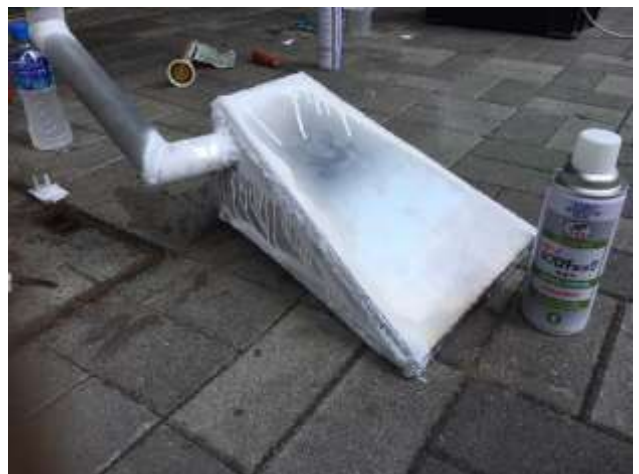
図 14 Fuel tank prototype spill check
